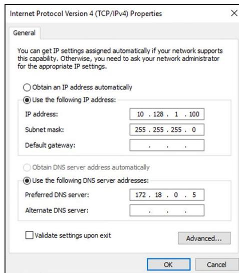
The second adapter is connected to the management virtual LAN configured within the hypervisor. This network card is configured to use a unique static IP address on the management network and does not have a default gateway configured.
