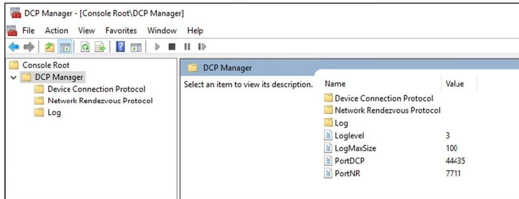
The DCP service is configured with ordinals 5 and 8 (or 14). The host addresses used are the IP addresses reserved for these services on the external network. The standard port for NCE is used.
